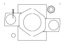
\$Ž? & Load Wiring 2-M4 #ž\$Ž\$@ž\_ \$Ž'@ž\_ ? Sj Torque 1.2-2N.m 2.0N.m Max
