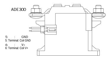
1+ Load Output Connected to Positive Pole (1+) 2-Load Output Connected to Negative Pole (2-)
